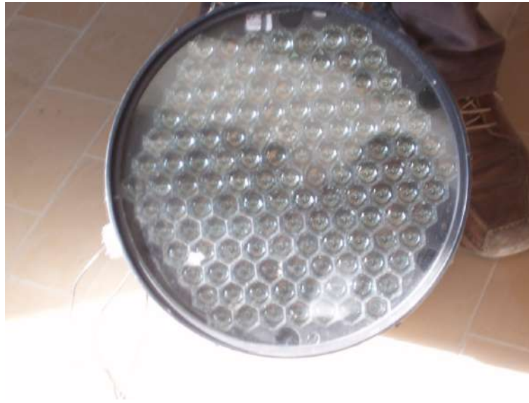
Figure 3.3: The front plate of the CT1 camera. In front of PMTs are the Winston cones – designed to minimize the dead-space between the photocathodes of the PMTs. Picture by Nikola Godinović from Split.
