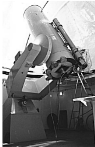
Figure 3.6: KVA-60 optical Cassegrain telescope located at ORM on La Palma. Source: http://www.astro.utu.fi/telescopes/60lapalma.htm
